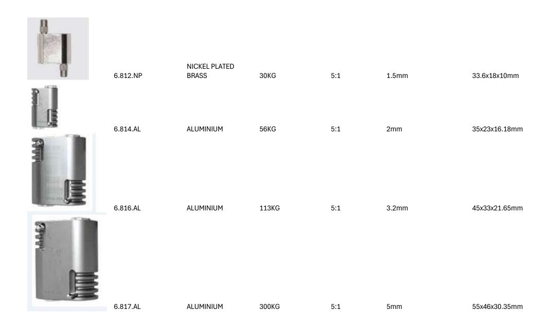
Only to be used with 7x7 or 7x19 Wire Rope Suspension Cable
